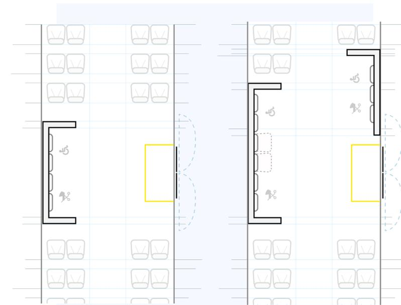
Could the bus have multiple spaces for wheelchairs? One in the front of the door and one with a seat with the back against driving direction
