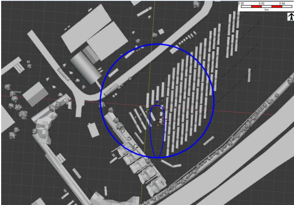
Figure 8.2 Max cloud footprint (shape and effect zone) for large releases from the hose to the connection unit A at a height of interest of 1 m. The concentration of interest is equal to LFL, at 8D wind conditions.
