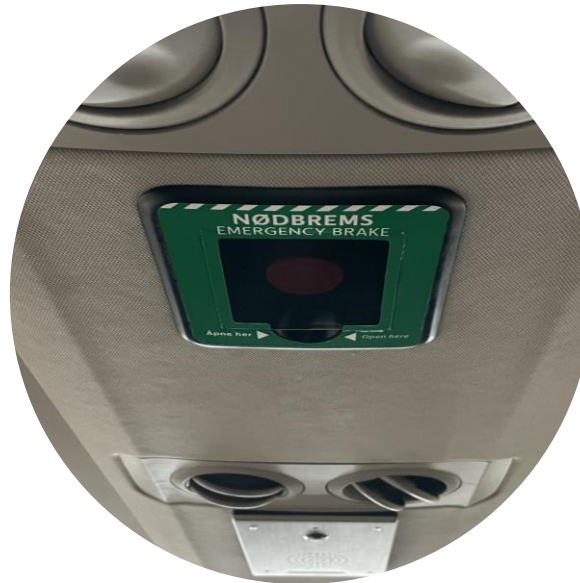
Emergency break/ stop buttons
